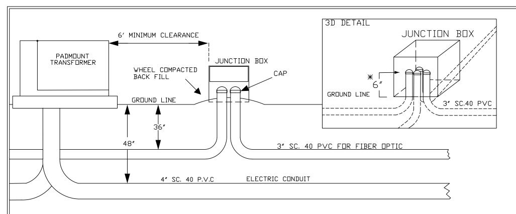
\*All 3" Conduit for Fiber Optic Communications will be Stubbed up 6" above grade level and capped off.
