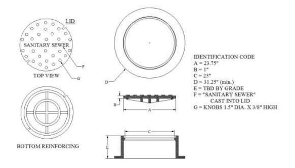
Figure 20 - Sanitary Cast Iron Lids, PST # 2501
