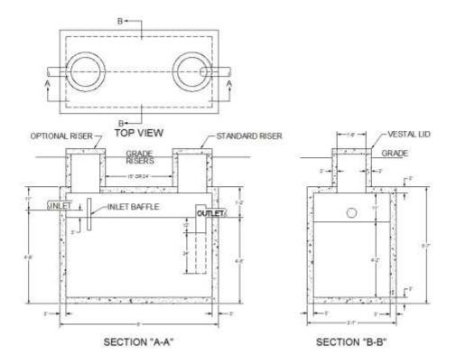
Figure 18- 500 Gallon Grease Trap, PST # 2401A (1 of 2)
