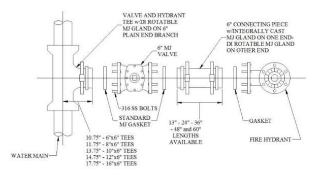
Figure 1- Mechanical Joint Fittings # PST 501A
