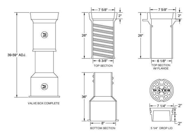
Figure 8 - Screw Type Valve Box Detail, PST 1301
