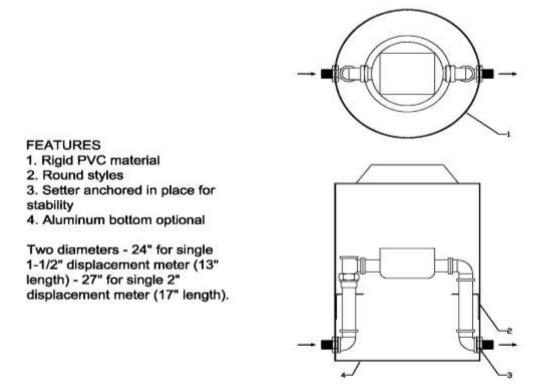
Figure 15 – Meter Pit Drawing, PST # 2250
