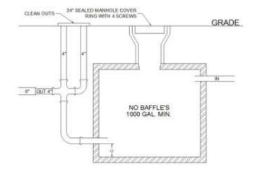
Figure 19 – Grease Trap Interceptor, PST # 2401 A (2 of 2)
