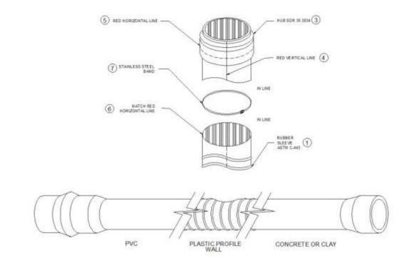
Figure 22 –Sewer Pipe Inserta-Tee, PST # 2801
