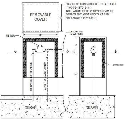
ALTERNATE COMPOSITION/STYLE SHALL BE THE MUELLER SINGLE COIL METER PIT MADE OF VINYL CHLORIDE PLASTIC (SEE ATTACHMENT "NOTES").
